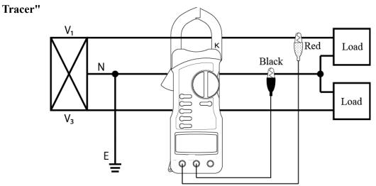
Connecting Method for 3 phase/3 wires(Measuring Mode: A) [Ld] is displayed on "Multi-Tracer"
