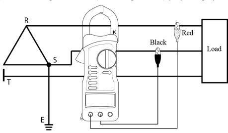
Connecting Method for 3 phase/4 wires Neutral point grounding(Measuring Mode:Y) [Ld] is displayed on "Multi-Tracer"
