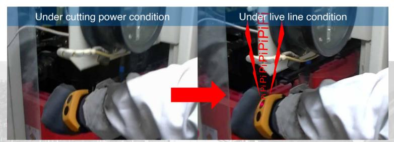
Voltage detection alarm with beeping and flashing
