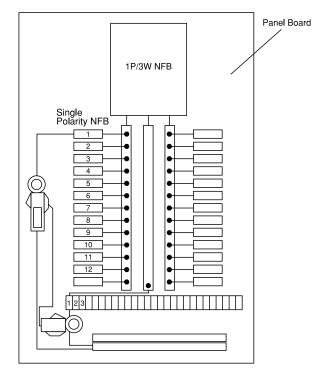
Model 2002 can measure load and leakage current by general method in the same manner as ordinary clamp meters but also can detect leakage current by using 2CT method in combination with optional CT sensor even in the fields where CT cannot be clamped to two wires in the single phase system.
