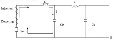
At the time of resonance by L & C0, current I will flow as the above route and can measure Re (Earth Resistance).
