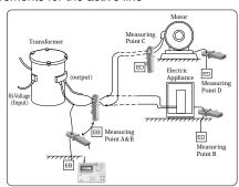
The earth resistance can be measured by clamping 2 CTs near at transformer (point A or B) and near at the electrical loading part (motor, electric appliance, etc.)
