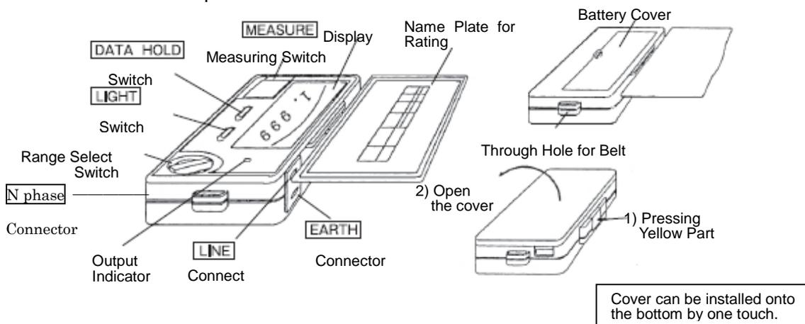
DATA HOLD : The displayed data on LCD is held by pressing this switch during measurement of insulation resistance and it will be released by pressing switch again.
