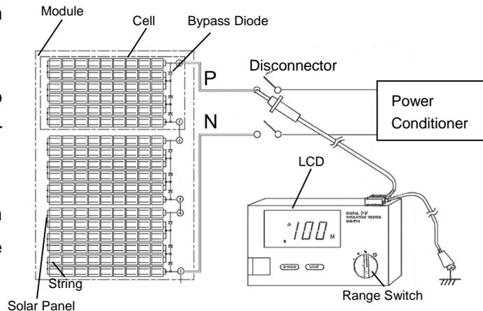
4) Connect EARTH lead of MIS-PVS with the earth terminal of PV system.
