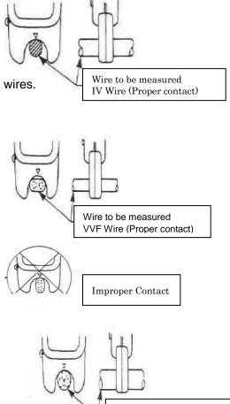
③ In the condition of ②, rotate the instrument about the wire to be measured and read the maximum indication value.
