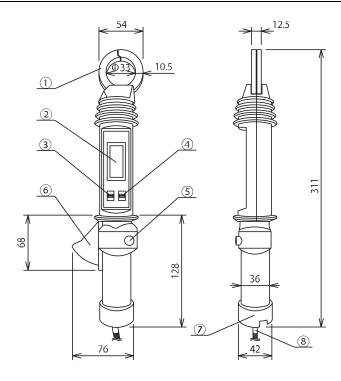
① Clamp CT : CT sensor detecting the current by clamping method. ② Open/Close Guide for CT : Clamping/releasing CT to or from the conductor by
